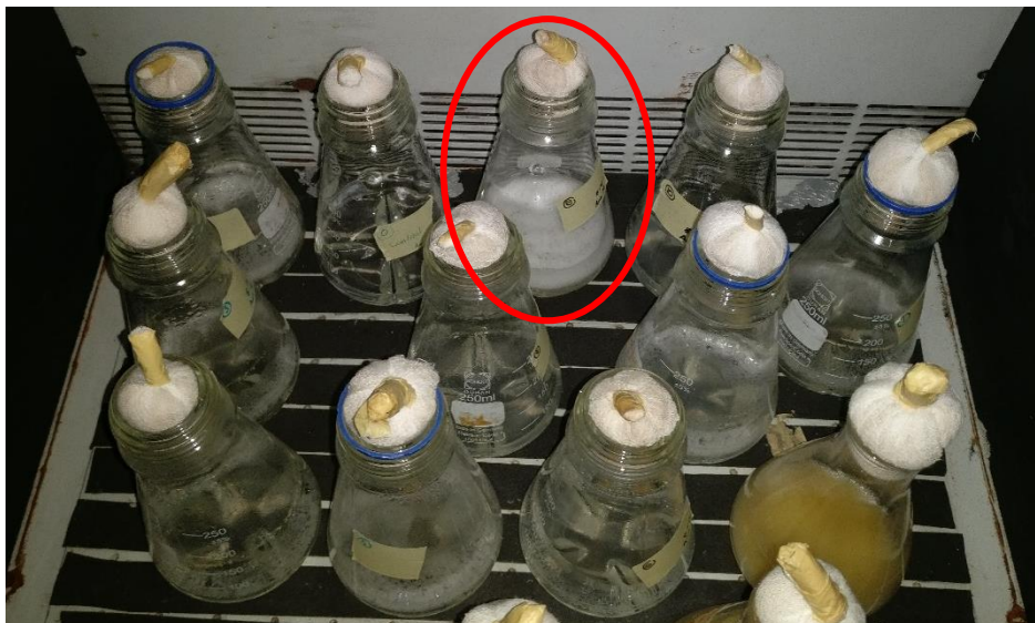
Figure 32 -Foam presence in some of the alkane bioremediation shake-flasks at day 6.
